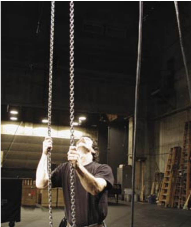
Figure 11. Rigger checking overhead chain
